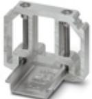
End clamp, for end support of UKH 50 to UKH 240, is pushed onto DIN rail NS 35 and fixed with 2 screws, width: 10 mm, color: aluminum
