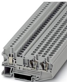
Feed-through terminal block, connection method: Spring-cage connection, Screw connection, cross section: 0.08 mm<sup>2</sup> - 6 mm<sup>2</sup>, AWG: 26 - 10, width: 6.2 mm, color: gray, mounting: NS 35/7,5, NS 35/15
